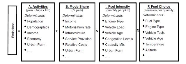
Figure II-1, Factors under the ASIF component
