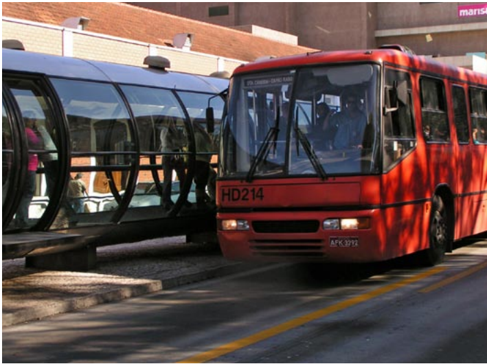
Figure 55 ▲ A high level platform like this one in Curitiba reduces boarding time, and so bus travel time. Photo by Manfred Breithaupt, Curitiba (BR), 2006
