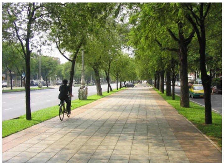
Figure 28 A wide pedestrian path on the median in Bangkok has trees to separate from car traffic and also provides shade to keep users cool.
