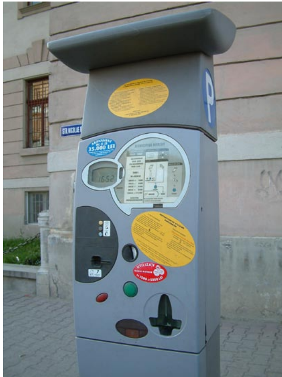
Figure 67 Solar-powered electronic parking meter for on-street parking.
