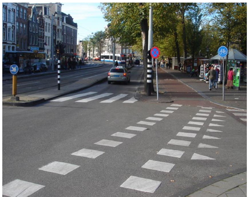
Figure 79 Multi-modal road design in Amsterdam. Roadway space is divided into separate right-of-way for tram, car, bicycle, and pedestrian.
