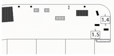
boxes, bus stands, telephone booths, stairways, poles) reduce the 'effective' width to, in this case 1.4m and 1.5m.
