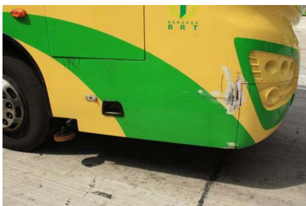
Figure 17: Damaged side of a BRT bus due to incorrect turning radius at one of the BRT terminals
