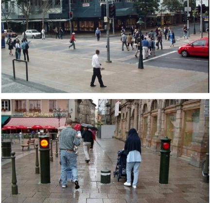
Figure 5 Concealable barrier for cars at the entrance to a car free zone, Strasbourg. Source: GTZ 2003
