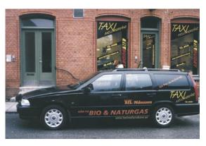
Fig. 1-11 Biogas driven taxi, Volvo, in Eslöv, Sweden
