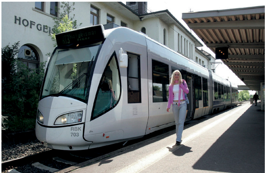
Figure 13 RegioTram as a dual-system or hybrid vehicle used on both city light-rail and regional rail lines within the Nordhessischer Verkehrsverbund (NVV).
