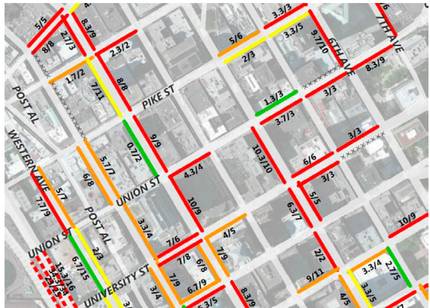
Fig. 94: Mapped results of an occupancy survey of on-street parking in part of Seattle's commercial core on a weekday in 2013. © Sightline Institute — Image from a report by Seattle's Department of Transportation is via the Sightline Institute, http://daily.sightline.org/2013/09/27/theres-a-place-for-us
