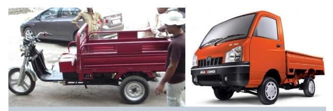
**Fig. 39a, b:** *E-tricycle as transport vehicle and the electric light lorry Maxximo.* © SIKCO, 2015; Mahindra, 2015
