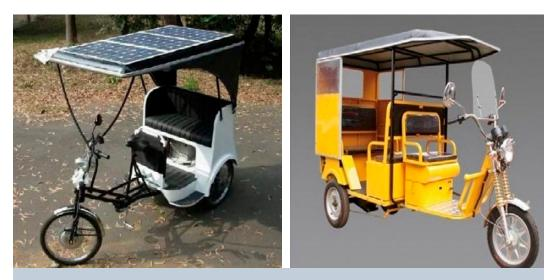
Fig. 37a, b: Tricycles with solar roof, being used as rickshaw. © SIKCO, 2015
