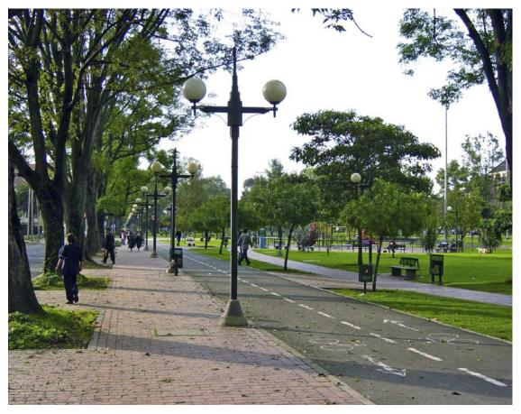
Figure 90 Public lightning of bicycle tracks and footpaths is essential to feel comfortable and safe after dark. Notice that in this situation the sidewalk has been combined with a cycle path. This is an effective way to enhance both cycling and walking, without creating an unnecessary conflict between cyclists and pedestrians.
