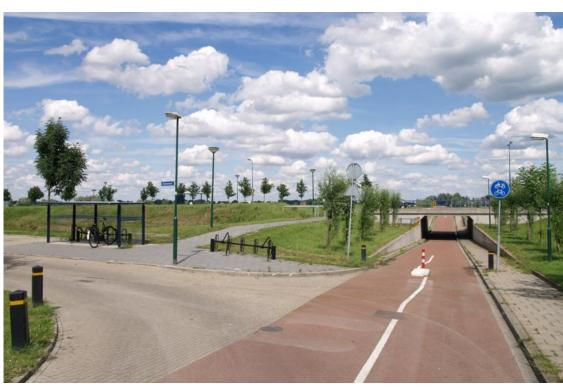
Given a choice, it is best to keep pedestrians and cyclists on ground level, while raising or lowering the metropolitan highway, not only because slopes and detours are less bothersome to motorized traffic, but also to enhance safety. Building this sort of highway is more expensive, but the additional cost of pedestrian/cycle facilities will be marginal.
