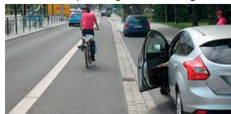
Sufficient safety clearance between parking lane and cycle lane (source: Tomas Cach)
