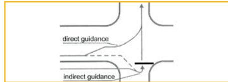
Direct and indirect intersection treatments for left-turning cyclists (source: FGSV (2010), p.39)
