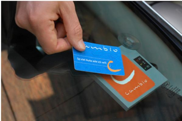
**Figure 8:** RFID card access to a carsharing vehicle.
