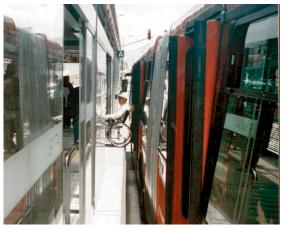
passengers have a greater tendency to depart the vehicle one-by-one when a gap exists between the vehicle and the platform. The flip-down ramps utilised in Curitiba and Quito avoid these cumulative customer hesitancies that will slow boarding and alighting. With the ramps customers will tend to move with greater confidence and speed.
