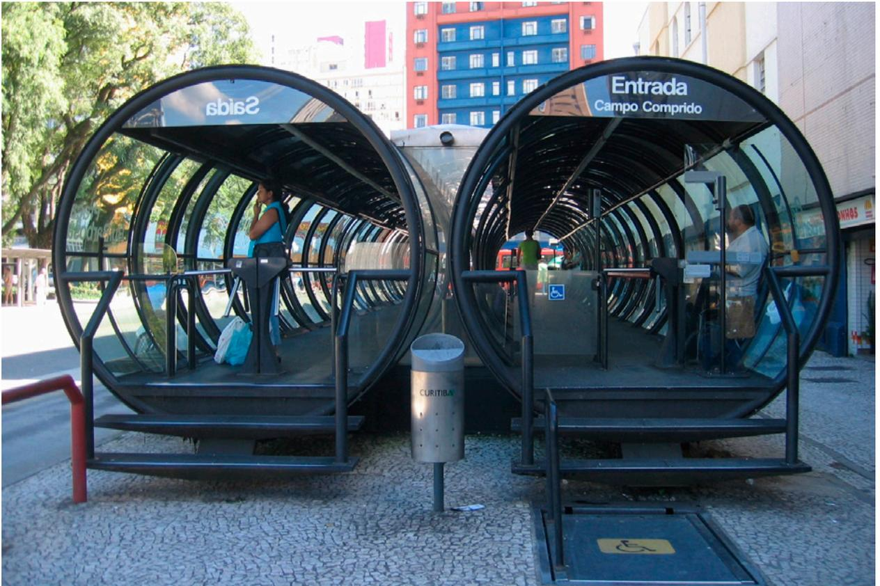
**Figure 35:** Elevated BRT station protects passengers from weather influences and contributes to safety aspects in Curitiba, Brazil.
