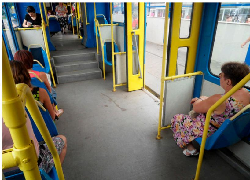
**Figure 53:** Tram modernisation is often a cost-efficient alternative to the procurement of new vehicles. The figure shows a refurbished tram with level-access entry operating at a Kiev tram system. © Mathias Merforth 2012
