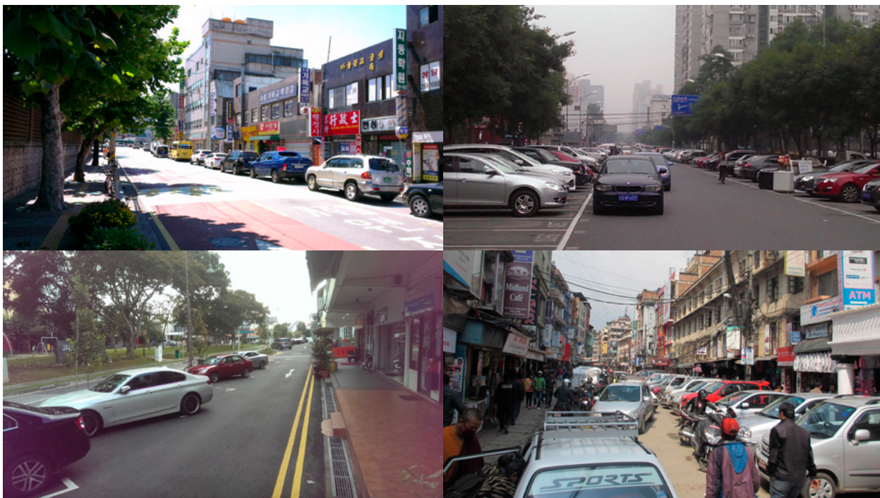
Fig. 30, 31, 32, 33: Parking orientations: parallel (top left), perpendicular (top right), angled (at an unusual 30°) (bottom left), perpendicular without markings (bottom right). © Paul Barter
