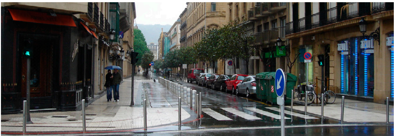
Fig. 50: Example of design that prevent or discourage nuisance parking in a self-enforcing way in San Sebastian, Spain. © Andrea Broaddus from SUTP on Flickr
