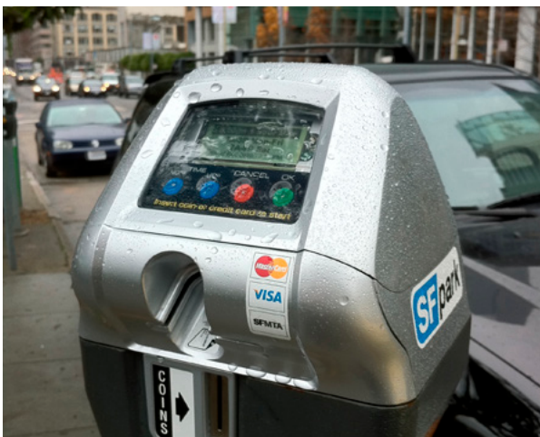
Fig. 67: Examples of modern digital on-street parking pricing mechanisms: Smart (digital) single-space meter in San Francisco. © Carlos Gomez on Flickr
