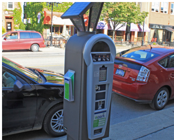
Fig. 68: Smart (digital) multi-space meter in Ann Arbor. © Dwight Burdette via Wikimedia Commons
