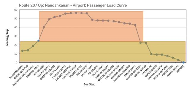
Figure 7: Passenger Load Curve of Route 207
