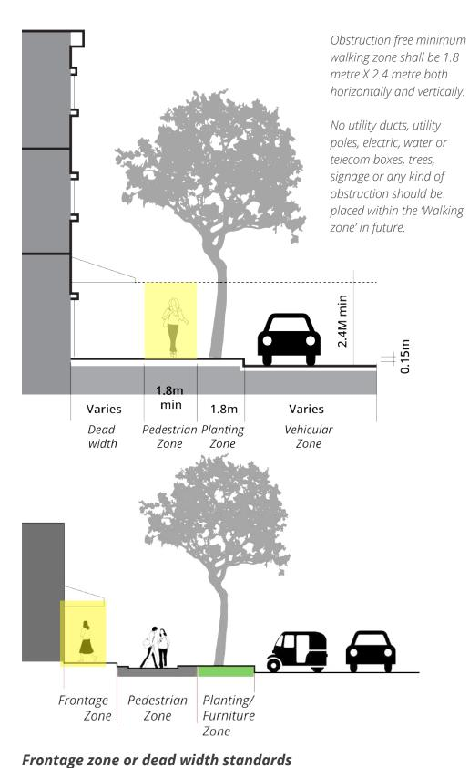
For footpaths in shopping area, an extra one metre should be added to the stipulated 4 metre width. In other situations where footpaths pass next to buildings and fences, a dead width of 0.5 metres can be added.
