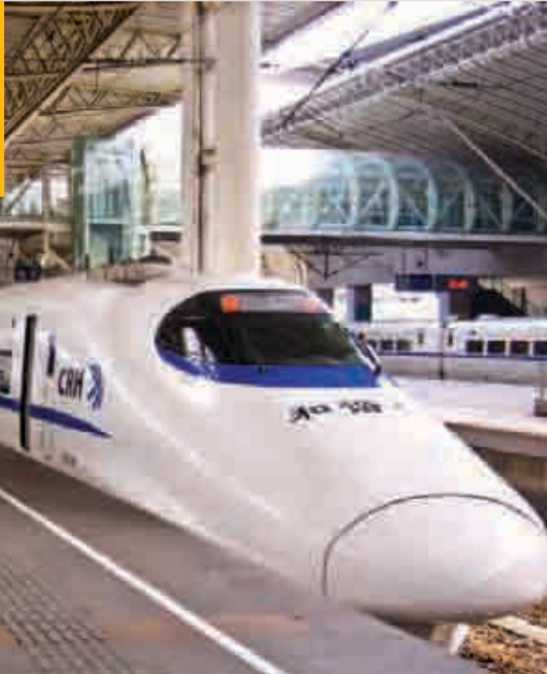
3.46. BEIJING (PRC) The bullet train from Beijing to Tianjin opened in 2008, with a line distance of 117 km and trains running at a maximum speed of 350 km/h. It takes just 30 minutes, giving people more choice in where they live and work. However, improved services can also induce new long-distance travel, making energy consumption a problem.
