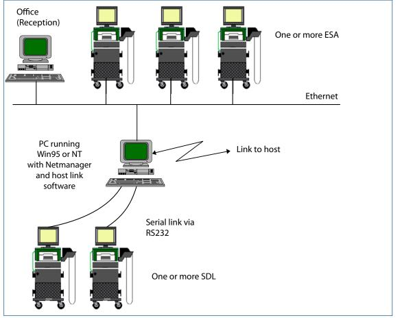
Fig. 38 Centralised survey system.
