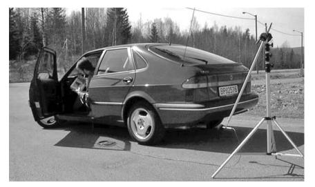
Fig. 33 Sound level measuring installation. Norsonic
