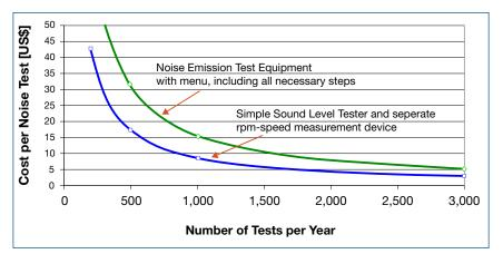
Fig. 32 Noise test cost varies according to equipment costs and the number of tests per year. stationary condition of the vehicle and there is no running or distance covered.
